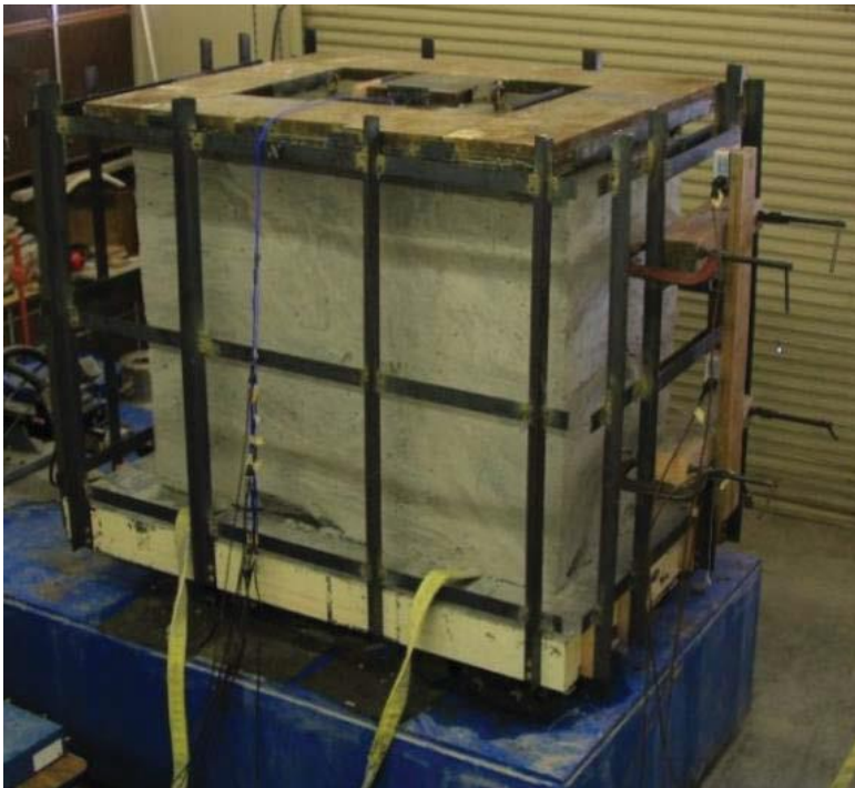
Figure 28: Geo-grid reinforced LCC block tested by Tiwari et al. (2018c and 2018d) on shake table, tested at surcharge pressure of 1.16 psi (copied from Tiwari et al., 2018c and 2018d)
