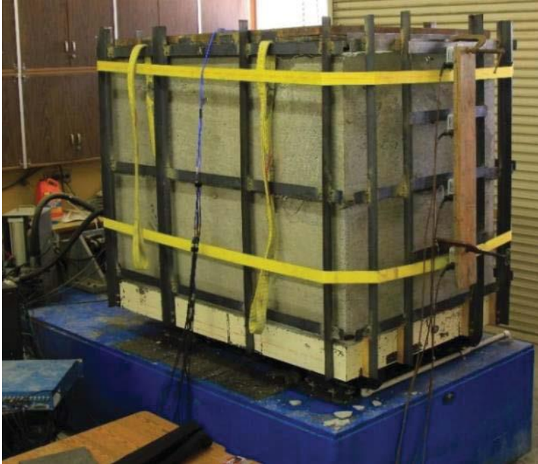
Figure 27: Geo-grid reinforced LCC block tested by Tiwari et al. (2018c and 2018d) on shake table, tested at surcharge pressure of 0.72 psi (copied from Tiwari et al. 2018c and 2018d)
