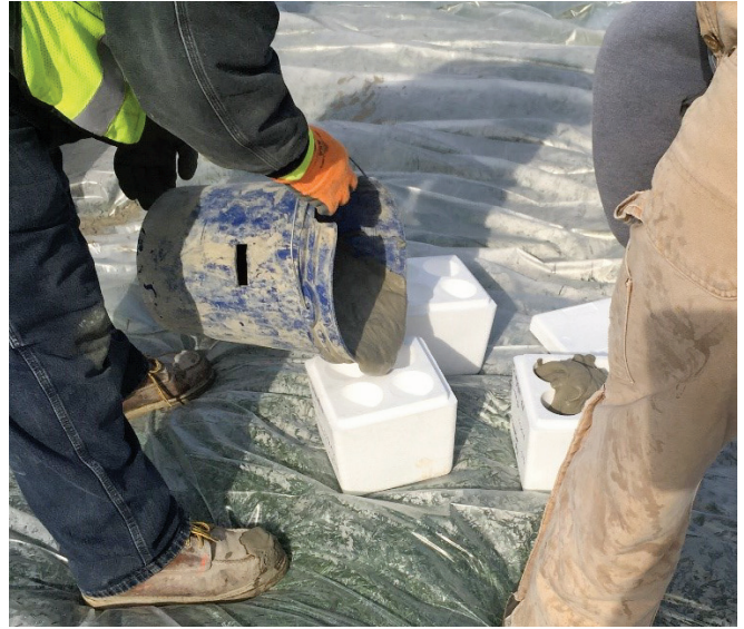
Figure 6.1. Sampling/testing LCC in the field (Michigan)
